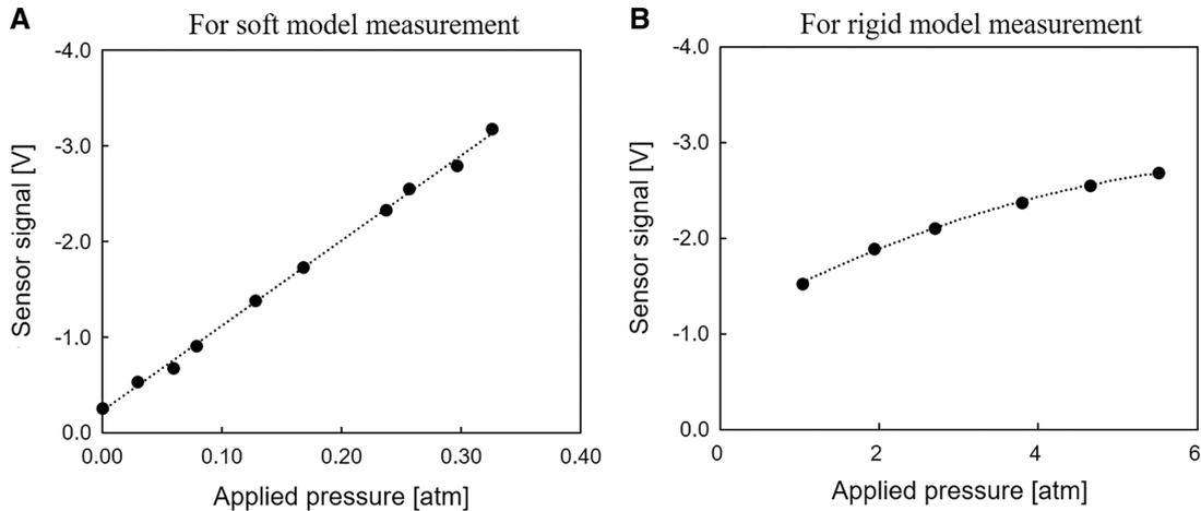
**Fig. 3** Calibration curves' contact pressure and output voltage for the film-type sensor. (A) Relationship in the low pressure range for soft model measurement and (B) relationship in the high pressure range for rigid model measurement.
