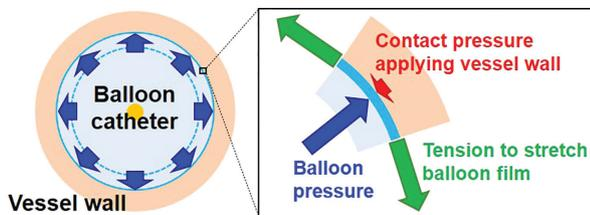
**Fig. 6** Schematic of the force relationship of circumferential cross-section during balloon dilation. Balloon pressure is not applied directly on the blood vessel wall because it first acts as a tensile force to stretch the balloon film.
