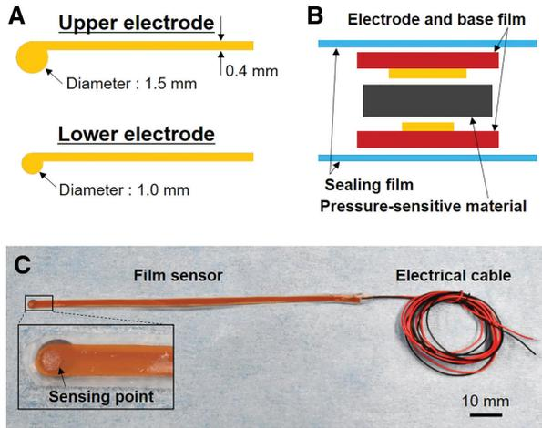
**Fig. 1** Film-type pressure sensor. (A) Upper and lower electrode structures, (B) schematic cross-sectional view of measurement points, and (C) sensor film after assembly.
