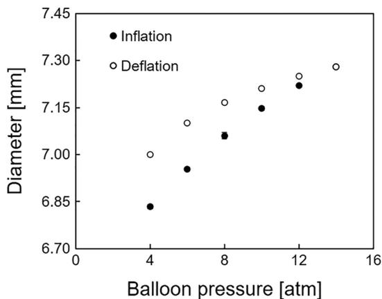
**Fig. 4** Compliance chart of the PTA balloon used in this study. The data (n = 3) are shown as mean (plot) and standard deviation (bar). PTA: percutaneous transluminal angioplasty
