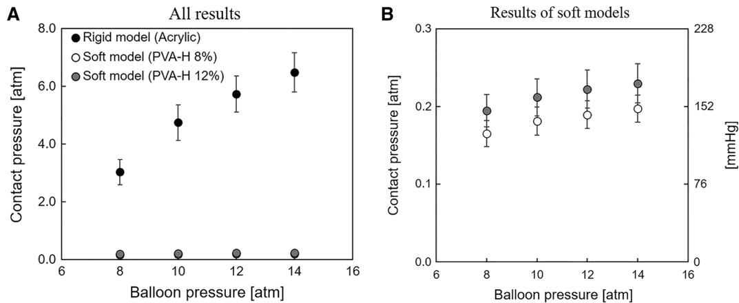
**Fig. 5** Relationships between the balloon pressure and contact pressure applied to the model vessel. The data (n = 9) are shown as mean (plot) and standard deviation (bar). (A) and (B) depict the same data with different contact pressure ranges.
