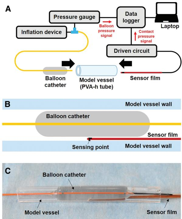
**Fig. 2** Contact pressure measurement during balloon dilation. (A) Schematic of measurement system, (B) schematic longitudinal section view of the inside of the model vessel, and (C) photograph of the model vessel setup during balloon dilation.
