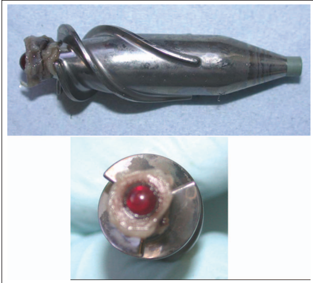
Figure 1. Frontal and lateral views of the impeller: visible thrombus around the ruby bearing.
