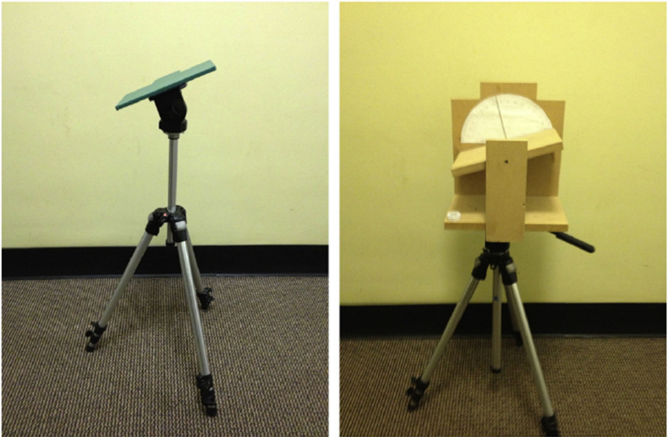
Fig. 4. Two palm boards used by Durgin, Hajnal, et al. (2010). At left is shown the simple palmboard (PB1) used in the demonstration Experiments 1 and 2 of Durgin, Hajnal, et al. (2010; it was also used by Durgin, Ruff, et al. (2012), Experiment 2). The head of the tripod served as the axis of rotation; the tripod head must be somewhat frictional to hold its position when set. At right is shown the low-friction palm board (PB2) used in Experiment 3 of Durgin, Hajnal, et al. (2010; it was also used by Durgin, Ruff, et al. (2012), Experiment 1, and by Li & Durgin, 2011). The axis is through the center of the palm board and the surface can be rotated effortlessly. Hand orientation can be read to 0.5^\circ from the protractor, or to 0.1^\circ by attaching a lightweight inclinometer or lightweight motion-capture equipment (Vicon) as used by Durgin, Hajnal, et al. (2010).
