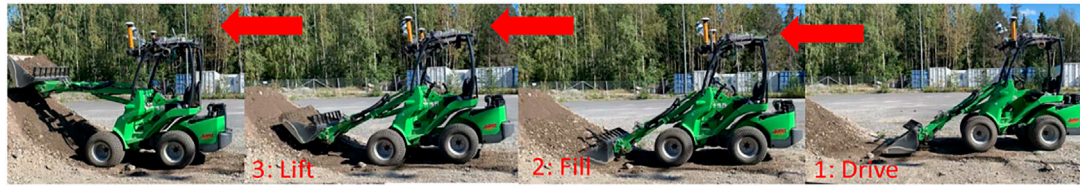
FIGURE 2 | Example of the typical stages in the pile loading task.
