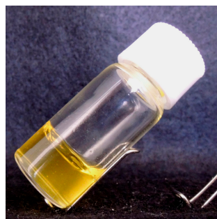
Figure 7. Formation of acrylamide hydrogel by using acyloyled polyNIPAM as a cross-linker ([cross-linker]:[acrylamide]:[APS]:[TEMED] = 2.5:2500:5:50 (molar base)).
