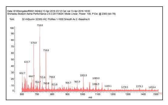
**Figure 3.** MALDI-ToF spectrum of the reaction of catechin with hexamethylene diamine at 185  $^{\circ}$ C, NaOH-catalysed. Range 600–1500 Da.
