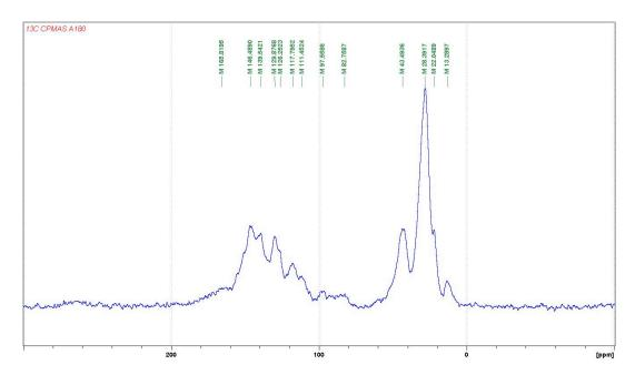
**Figure 16.** Cross-polarisation/magic-angle spinning (CP-MAS) <sup>13</sup>C NMR spectrum of the reaction of catechin with hexamethylene diamine at 185 °C, *p*-toluenesulfonic acid (pTSA)-catalysed.
