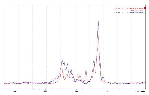
**Figure 20.** Superposition for comparison of the CP-MAS  $^{13}$ C NMR spectra of the reactions of catechin with hexamethylene diamine at 185  $^{\circ}$ C (blue curve) and at 100  $^{\circ}$ C (red curve), both pTSA-catalysed.
