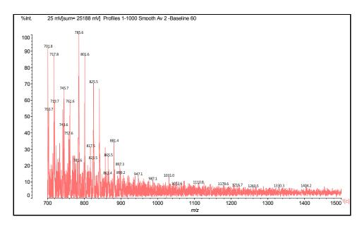
**Figure 23.** MALDI-ToF spectrum of the reaction of mimosa tannin extract with hexamethylene diamine at  $100 \,^{\circ}$ C, pTSA-catalysed. Range  $700-1500 \, \text{Da}$ .
