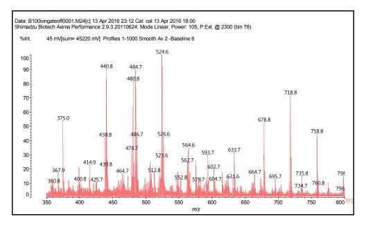
**Figure 2.** MALDI-ToF spectrum of the reaction of catechin with hexamethylene diamine at 185 °C, NaOH-catalysed. Range 350-800 Da.
