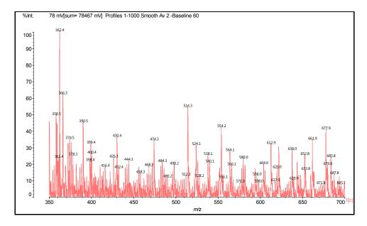
**Figure 22.** MALDI-ToF spectrum of the reaction of mimosa tannin extract with hexamethylene diamine at  $100 \,^{\circ}$ C, pTSA-catalysed. Range  $350-700 \, \text{Da}$ .
