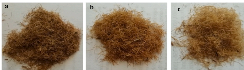
Fig. 3. Real photos of (a) Raw PO fibers, (b) KOH treated PO fibers and (c) H 3 PO 4 treated PO fibers.
