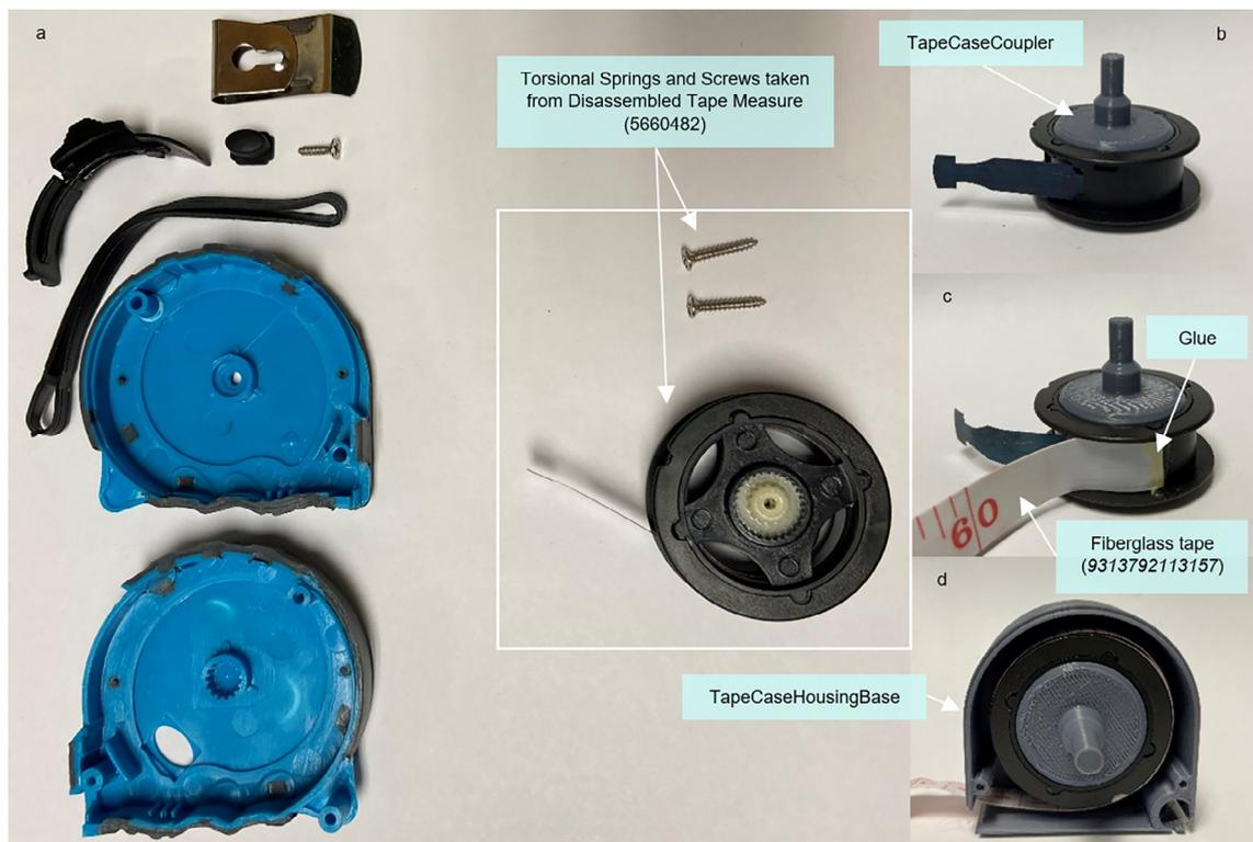
**Fig. 4.** (a) Disassembly of tape measure, (b) insertion of coupler, (c) attachment of fiberglass tape, and (d) insertion of barrel into base of tape measure housing.
