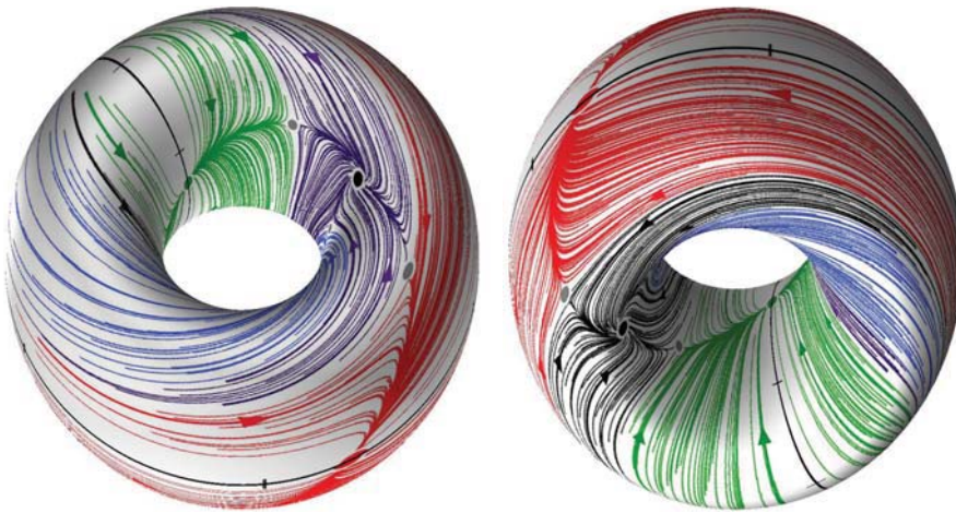
Figure 5. Poincaré return maps depicted on the torus. The return maps for the phase lags \{\Delta\phi_{21}^{(n)}, \Delta\phi_{31}^{(n)}\} between homogeneous cells at 50% DC correspond to trajectories on a 2D torus [0,1) \times [0,1) . Different colors denote attractor basins of several FPs corresponding to phase locked states of distinct bursting rhythms. doi:10.1371/journal.pone.0092918.g005
