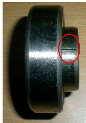
Figure 15. Physical photo of the N205 cylindrical bearing with outer ring defect.
