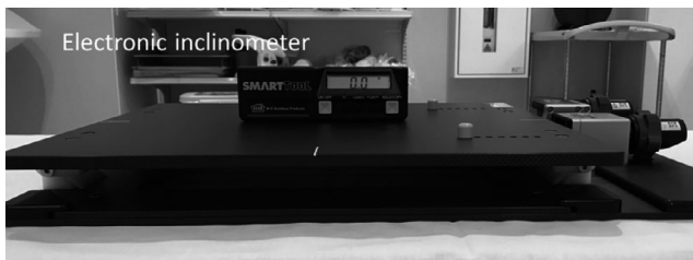
FIG. 3. Experimental setup for rotational motion accuracy measurement in pitch and yaw angles.
