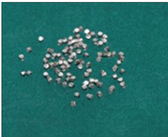
Figure 2: Stainless steel beads, generally used for embedding of pressure moulding models
