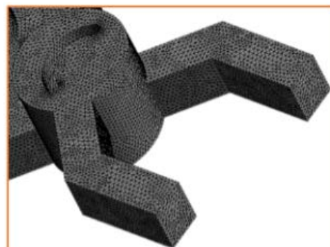
Figure 3. Structure of the generated mesh grid.
