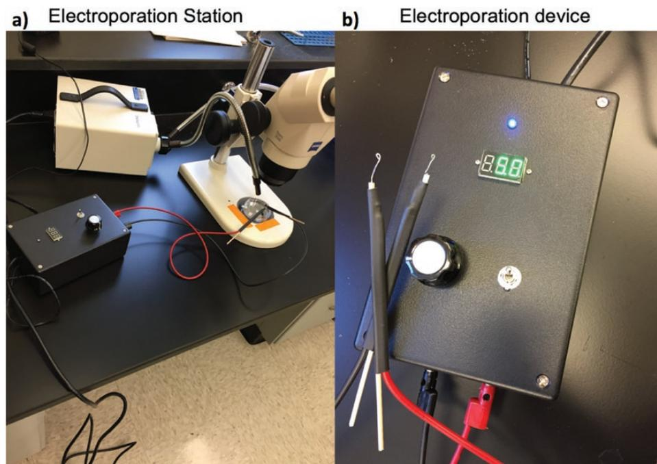
**Fig. 1.** Image depicting the electroporation station (a) and the electroporation device (b) used to introduce the CRISPR/Cas9 complex into aphid offspring in vivo.
