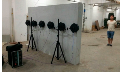
Figure 7. UWB MIMO radar system and the experimental scene.
