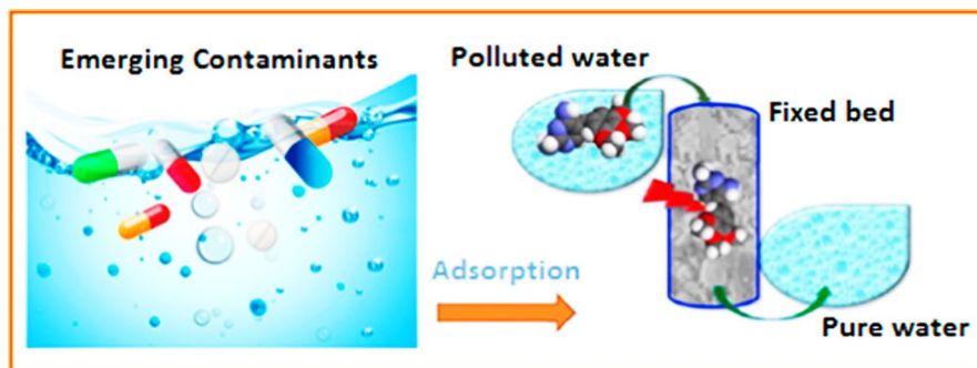
Fig. 5 Explanation of the sorption process on a fixed bed for effective removal of pharmaceutical contaminants. Reproduced with permission [109], Copyright 2018, Elsevier
