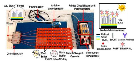
**Figure 5.** A microfluidic immunoarray with a 30-well detection array attached to PCB-controlled micropumps and sample/reagent cassette. The Arduino microcontroller is the microprocessor used to function the micropumps in order to perform the assay. Reproduced with permission from ref. [107]. Copyright 2015 American Chemical Society.
