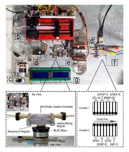
**Figure 10.** Illustration of an automated microfluidic immunoarray platform, featuring; (a) Arduino Uno microcontroller, (b) syringe pump, (c) sample injector, (d) servo-actuated valves, (e) capture chambers and magnetic stirrers, (f) detection chambers, and (g) LCD displays. Reproduced with permission from ref. [55]. Copyright 2019 Wiley-VCH Verlag.
