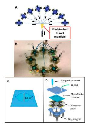
**Figure 11.** An electrochemical microfluidic immunoarray: (**A**) 256 individual working microelectrodes configuration; (**B**) 8 microfluidic immunoarrays are connected via miniaturized 8-port manifold; (**C**) molded PDMS microfluidic channel, and (**D**) deconstructed view of the integrated microfluidic immunoarray. Reproduced with permission from ref. [123]. Copyright 2016 American Chemical Society.
