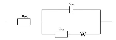
**Figure 13.** Randles equivalent circuit to the model the charge flow during electrochemical impedance spectroscopy detection, R<sub>CT</sub> represents the charge transfer resistance, R<sub>SOL</sub> denotes the uncompensated solution resistance, C<sub>DL</sub> represents the capacitance and W signifies the Warburg diffusion coefficient.
