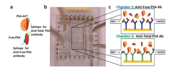
**Figure 14.** (a) Schematic representation of PSA antigens-related (cPSA and fPSA) and (b) device composed of two chambers for detecting the antigens: (c) one chamber is functionalized with anti-fPSA antibodies (Chamber 1) and the other one with anti-tPSA antibodies (Chamber 2). Reproduced with permission from ref. [129]. Copyright 2013 Royal Society of Chemistry.
