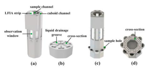
**Figure 8.** Detailed figure of the two types of multi-channel LFIA reaction columns; (a) Single-sample, multimarker reaction column (Type 1); (b) cross-sectional view of Type 1 LFIA column; (c) multisample, single-marker reaction column (Type 2); (d) Type 2 column's cross-sectional view. Reproduced with permission from ref. [114]. Copyright 2020 Elsevier.
