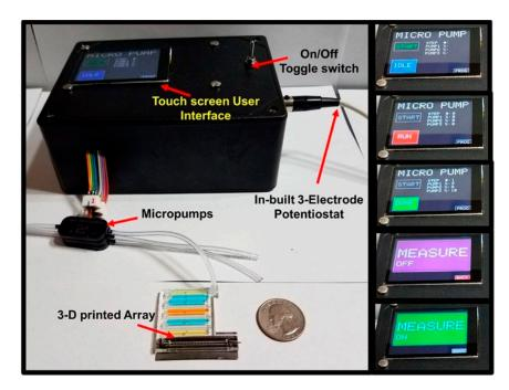
**Figure 7.** A 3D-printed immunoarray with touch screen user interface to control ECL measurements. A microfluidic array connected to a micropump is shown with dye-filled reagent chambers and graphite detection chip. Inset figures show multiple immunoassay steps along with messages to inform the user. Reproduced with permission from ref. [52]. Copyright 2018 American Chemical Society.
