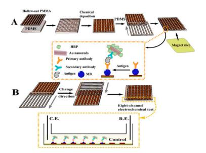
**Figure 12.** A flexible PDMS  $8 \times 8$  electrode immunoarray; (**A**) Schematic of preparing the microchip along with the sensor surface modifications; (**B**) Illustration of the detection of PSA, PSMA and IL-6, with control measurements, in one microchannel. Reproduced with permission from ref. [69]. Copyright 2014 American Chemical Society.
