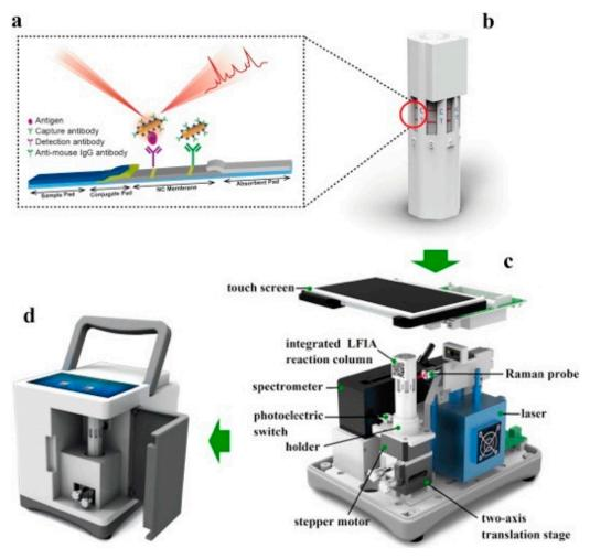
**Figure 9.** Illustration of portable SERS-based LFIA reader; (**a**) LFIA strip and (**b**) multi-channel LFIA reaction column, (**c**) Detailed schematic of the SERS-based LFIA reader and (**d**) the completed view of the portable reader. Reproduced with permission from ref. [114]. Copyright 2020 Elsevier.
