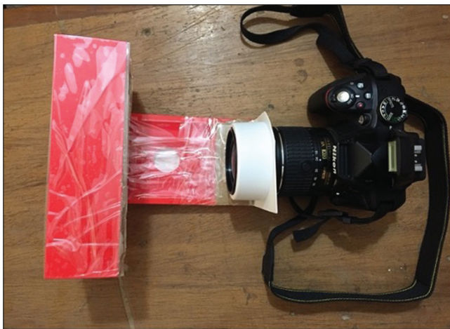
Figure 1: Digital camera with a frame providing a fixed object-lens distance
