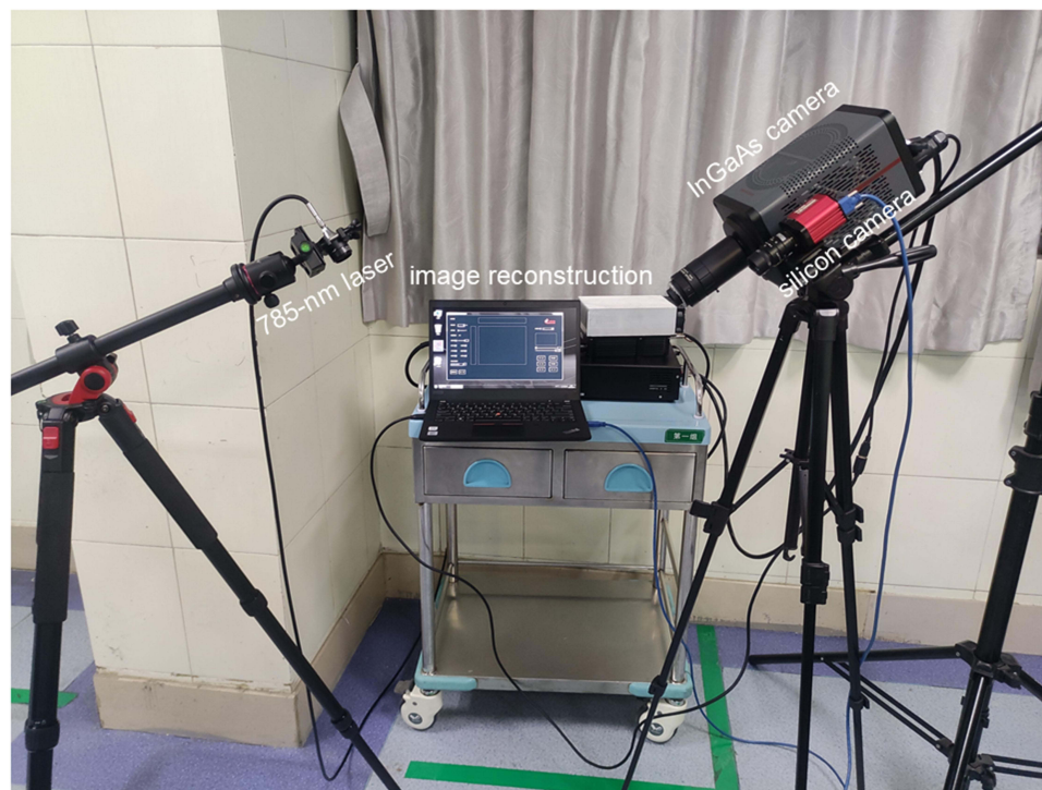
Figure 1 NIR-III fluorescence imaging system used for in vivo NIR fluorescence imaging in porcine limbs.
