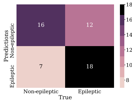
Fig. 10. Confusion matrix Model LOG-REG-01. From left to right and from top to bottom the number of true negatives, false positives, false negatives, and true positives.
