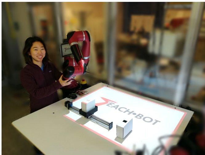
Fig. 1. The TeachBot System. A collaborative robot, a cloud computer (not shown), a projector (not shown), and peripheral devices.
