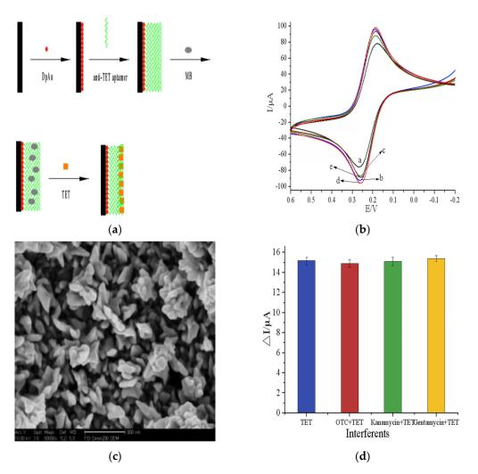
**Figure 4.** Methylene blue (MB)/anti-tetracycline (TET) aptamer/DpAu/glassy carbon electrode (GCE) immunosensor fabrication process (**a**), cyclic voltammograms (CVs) of different modification processes of GCE (**b**), scanning electron microscope (SEM) image of dispersed AuNPs over GCE (**c**), aptasensor specificity in the presence of different interferences (**d**). Reproduced from ESG [71].
