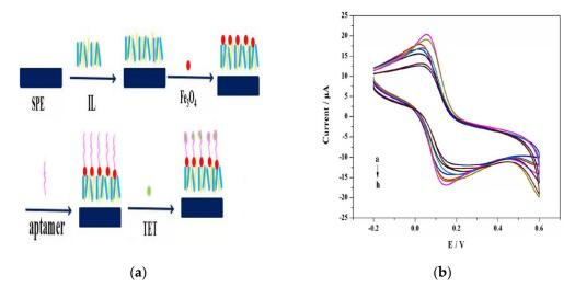
**Figure 6.** TET/Apt/Fe<sub>3</sub>O<sub>4</sub>/ionic liquid (IL)/screen-printed electrode (SPE) Aptasensor fabrication process (**a**), cyclic voltammograms of the aptasensor toward different concentrations of tetracycline (1.0 to 108 nM) (**b**). Reproduced from ESG [89].
