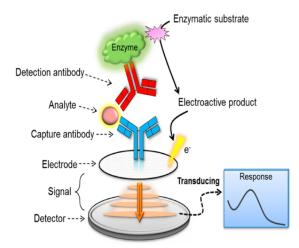
Figure 1. Electrochemical immunosensor basic analytical principle. Reproduced from MDPI [47].
