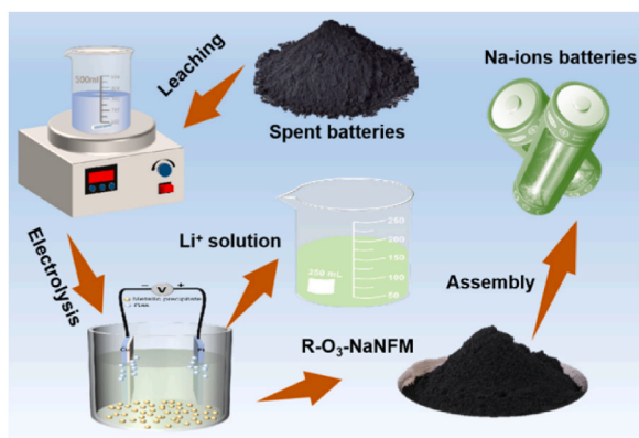
Fig. 1. Schematic diagram of the recycling of the spent LNMO material to the \text{R-O}_3\text{-NaNFM} .
