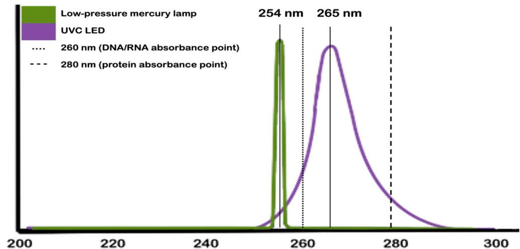
**Figure 1.** Wavelength peaks according to the UVC sources. Note: We abstained from providing the curve for medium-pressure lamps because they overlap with one of the UVC LEDs. For technical parameters about UVC traditional sources and LEDs, we suggest moving to Section 4.
