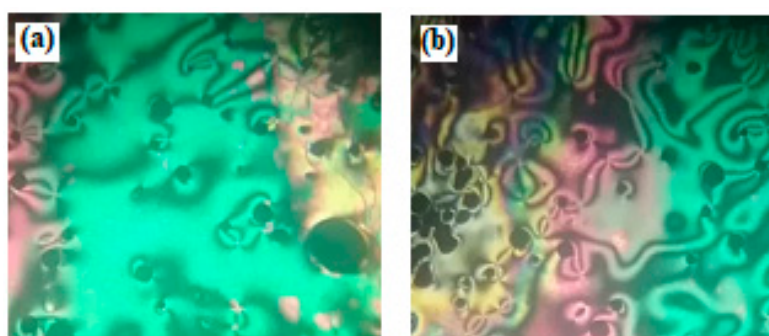
Figure 4. Nematic phase textures under polarized-optical microscopy (POM) of the supramolecular complexes (a) A10/I8 at 72.0 °C upon heating; and (b) A12/III16 at 77.0 °C upon cooling.
