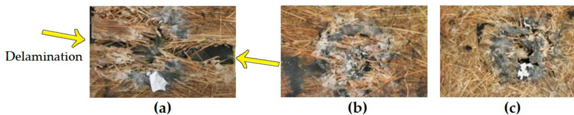
Figure 8. General macroscopic aspect after ballistic test of MAS targets with second layer of epoxy composites reinforced with 30 vol% of guaruman fibers: (a) continuous aligned, (b) cross-laid, and (c) short-cut randomly dispersed; all backed by 5 mm thick Kevlar™ panel.
