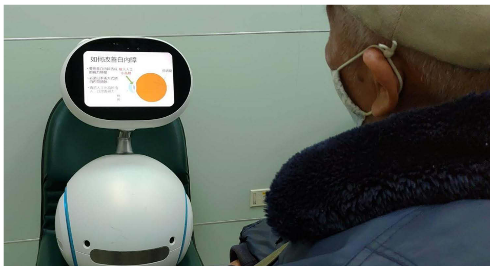
Figure 2 A participant underwent the decision-making process using the computerized patient decision aids on an interactive robot. The robot was equipped with a touchscreen, speakers, camera, and multiple sensors to interact with users. In the photo, the screen is explaining how the intraocular lens can treat the cataract via audio and graphic expression.
