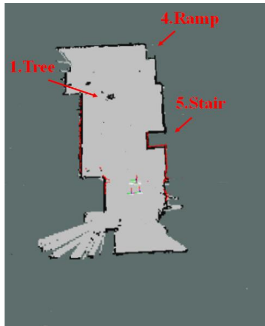
Figure 11. 2D map built using the LRF sensor.
