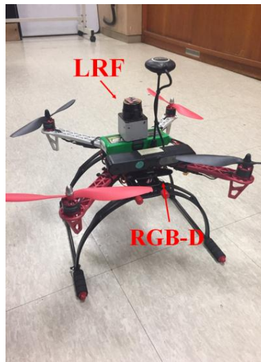
Figure 5. Aerial robot used in this study.
