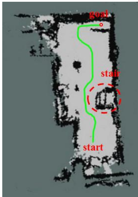
Figure 16. Mobile robot's navigation results using the topographical information of elevation map on the 2D grid map.
