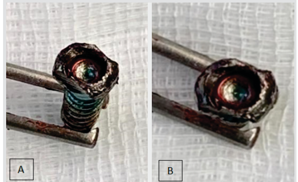
Figure 3: (a and b) Post-operative photographs of the extracted locking screw. Two sides of the screw head were burred off to create a more rectangular shape. The rest of the screw was observed to be structurally intact.
