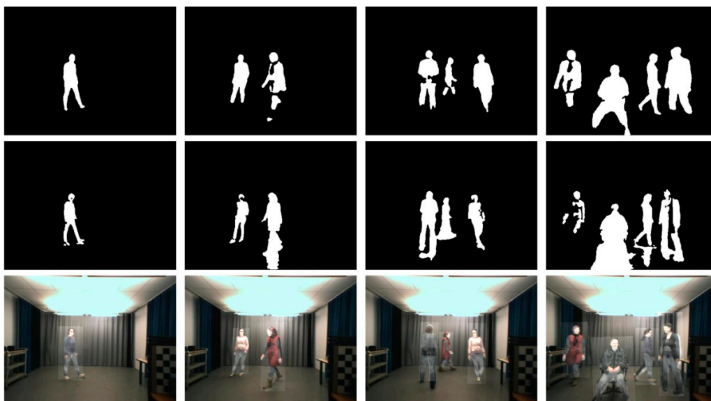
Figure 8. Noisy foreground frame pairs in the OTCBVS dataset and the registration results on these frames. The first row is infrared foregrounds and the second is visible foregrounds. The last row is the registration results on these pairs.
