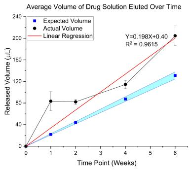
Figure 7. Validation of In Vivo Delivery Rate. The predicted flow rate (black line, circle markers) for osmotic pumps is plotted with the actual flow rate (blue squares in cyan band) for N=4 animals. A linear equation was fit to the measured data (red line), showing that the actual flow rate was 19.8  $\mu$ L/h with an R2 value of 0.9615. The expected flow rate is 13  $\mu$ L/h, plotted with a +/- 5% band, the expected acceptable error of the osmotic pump flow rates.
