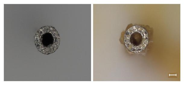
**Figure 8.** High Magnification Image of Explanted Cannula. The explanted cannulas seemed to show cellular debris and brain tissue on the inside of the cannulas, which may have caused the unstable drug delivery rate. Scale bar =  $100 \mu m$ .
