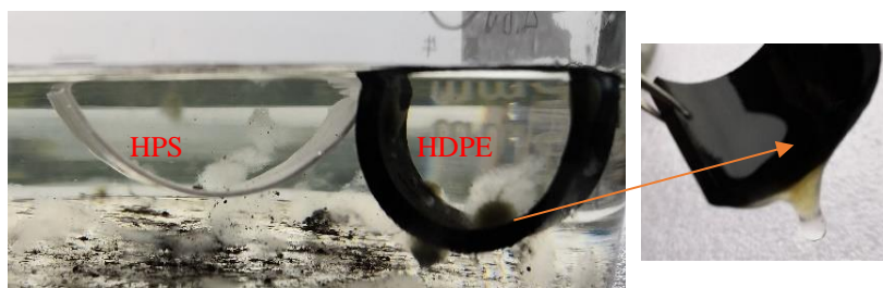
Figure 11. Material samples immersed in the simulated leachate (pH = 4.0).
