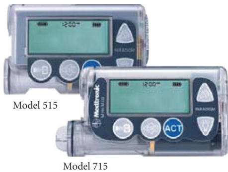
FIGURE 3: Another example of insulin pumps of Medtronic. A processing module has a small display that shows a current rate of an exogenous insulin infusion. It also has several control buttons just below the display. Two of these buttons are used to manage a current insulin infusion rate.
