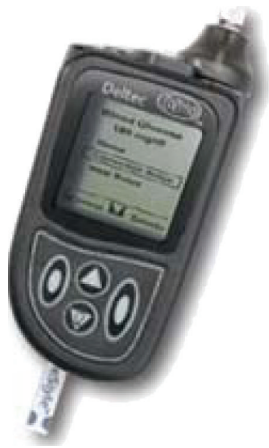
FIGURE 6: An image shows a fingerstick meter reading. In the use of the sensor, first off, cut the tip of a finger or earlobe bleeding. Then put the blood on a blood glucose sensor, which is a protuberance at the bottom of the module. The result is shown on the display in the middle-top of the module.
