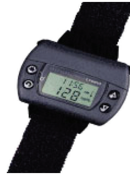
FIGURE 7: An image shows a list-watch type noninvasive blood glucose measurement [1]. The sensor can avoid damaging the tip of a finger or earlobe to sample blood in a noninvasive way. Therefore, it basically utilizes a quite low electric current to draw blood glucose penetrable through the skin. This sampled glucose is aggregated into a sensing part of the device integrating an electrode that is used for measuring blood glucose levels.
