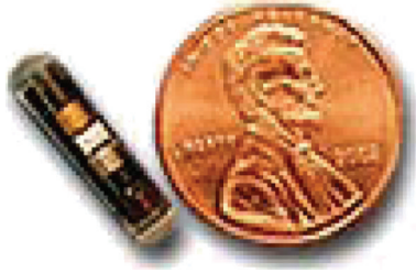
FIGURE 5: An image shows a miniature size of in vivo blood glucose sensor that is being developed [15]. It is currently proven by FDA that in vivo blood glucose sensors are only safe and reliable in a short period of time (e.g., three days). Thus after the period, they are required to be replaced by a new one regularly to keep their accuracy.
