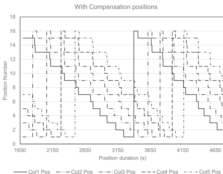
Figure 10. EBA-SMB experimental logged data describing the switching of eight columns in the presence of a compensation position.
