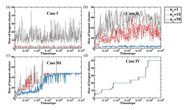
**Figure 5.** Time evolution of the size of the largest cluster size (number of bottlebrushes) in various solvents: (**a**)  $a_{sc-sol} = 78$  (Case I), (**b**)  $a_{sc-sol} = 83$  (Case II), (**c**)  $a_{sc-sol} = 84$  Case (III), and (**d**)  $a_{sc-sol} = 89$  (Case IV). Black dotted, red dash-dotted, and blue solid lines of the same color represent the number of contacts used to identify clusters ( $n_c = 1$ , 13, and 78, respectively).
