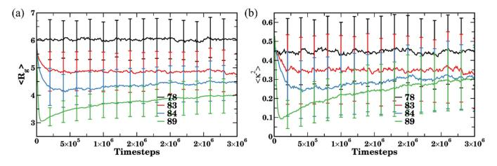
**Figure 8.** Time evolution of (**a**) radius of gyration and (**b**) shape anisotropy. At each time step, the data are averaged over all  $n_{MBB} = 77$  bottlebrushes in four independent simulation sets, error bars represent standard deviation. Black, red, blue, and green curves correspond to affinities  $a_{sc-sol} = 78$ , 83, 84, and 89, respectively.
