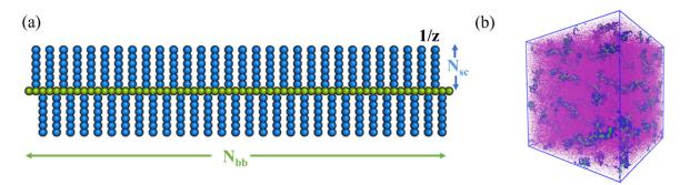
**Figure 1.** (a) Bottlebrush architecture, backbone (bb), and side chain (sc) beads are shown in green and blue,  $N_{bb}$  and  $N_{sc}$  denote numbers of beads within the backbone and side chain, respectively. (b) Initial distribution of  $n_{MBB}$  = 77 bottlebrushes equilibrated within the good solvent; solvent beads are shown in purple using reduced bead size.
