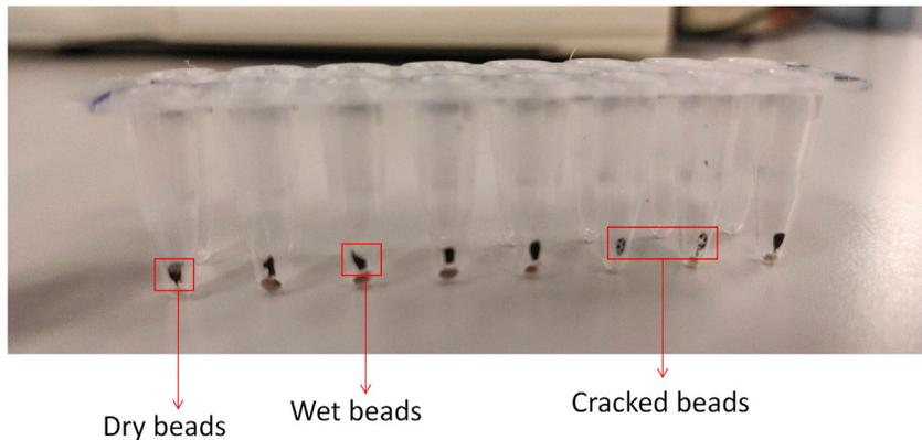
**Figure 10. Beads drying state**
