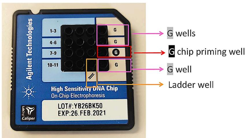
**Figure 13. Bioanalyzer 2100 dsDNA chip**
