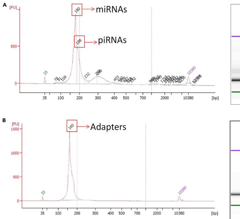
**Figure 18. Examples of successful and failed libraries electropherograms**
