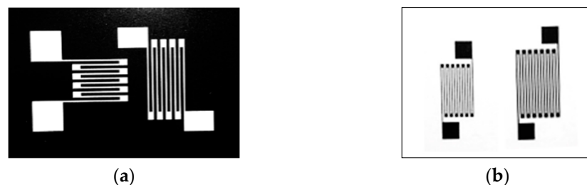
Figure 3. Photolithography process mask. (a) Film paper used in PMS. (b) Film paper used in PIBE.
