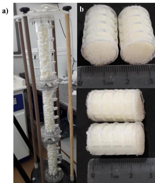
**Figure 1.** (a) Trickling filter filled with the support material before inoculation; (b) support media mini-BioBobs and their size in detail.
