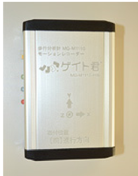
Figure 1. Portable gait rhythmogram (MG-M 1110, LSI Medience Corporation, Tokyo, Japan). Size = 8 \times 6 \times 2 cm. Weight = 80 g.
