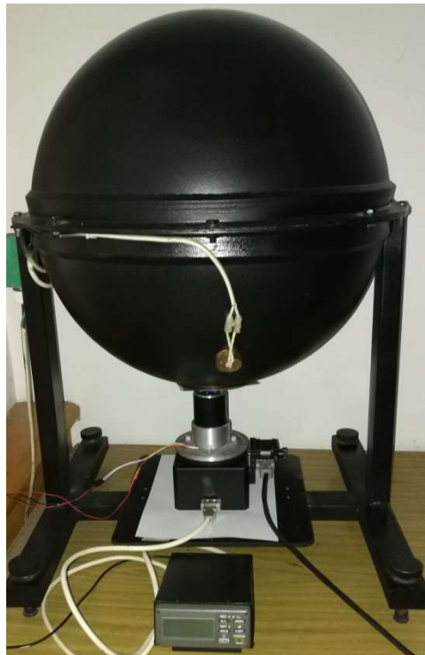
Figure 15. Photograph of indoor calibration setup.
