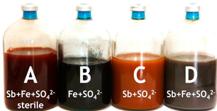
Figure 7. Bioreactors 21 d after inoculation: reddish-brown (A), black (B); dark orange (C); and charcoal gray (D).
