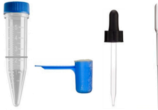
Figure 1. Sample preparation kit. From left to right, a sample tube with a marker line for 10 mL, a 1/2 tablespoon scoop, and an eyedropper or Pasteur pipette for sample deposition.
