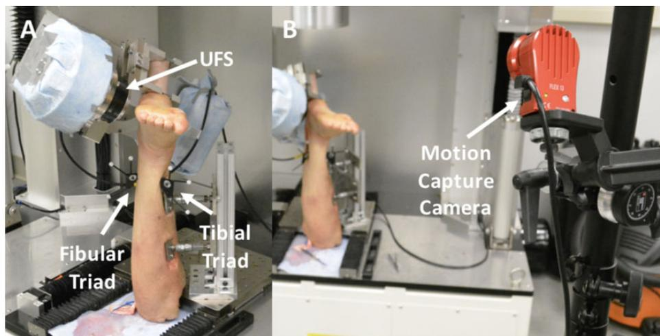
**Figure 2.** (A) Experimental setup with full-length fibular specimen rigidly mounted to the robotic testing system through the calcaneus and a universal force-moment sensor (UFS). Optical motion capture markers are noted on the fibula and tibia. (B) The experimental setup with the robotic testing system surrounded by 6 motion capture cameras, such as the one shown, arranged in a semicircular configuration.
