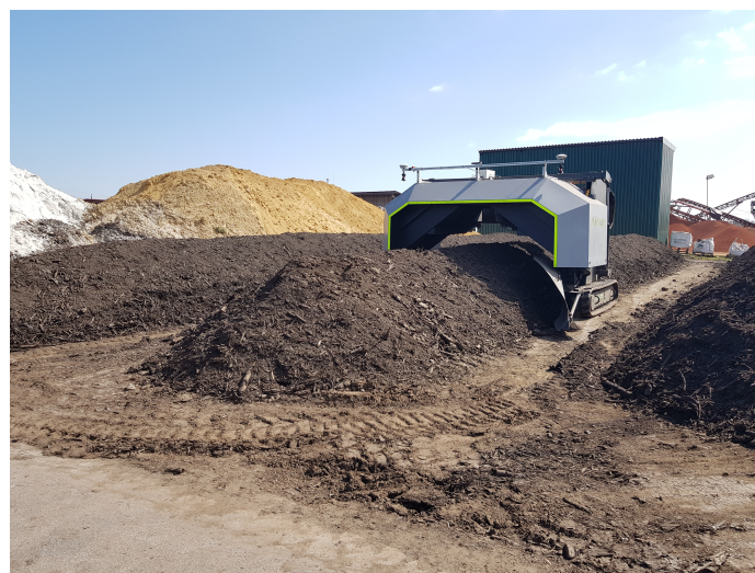
Figure 5. The tracked compost turner eWender E35eco during the field tests.
