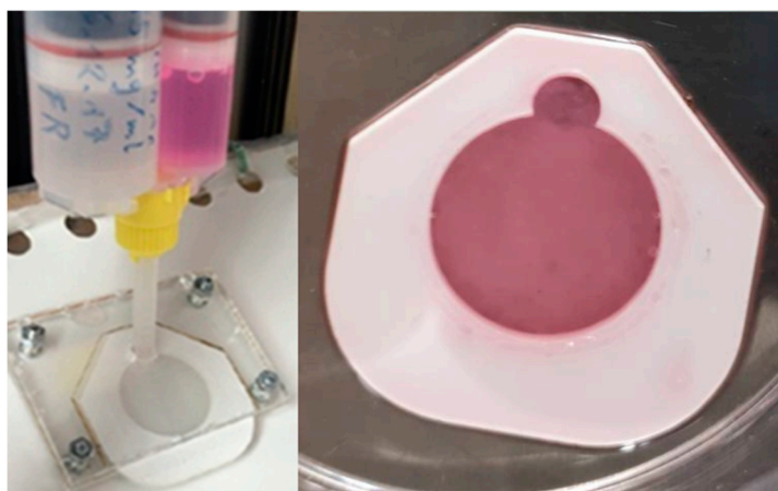
Figure 6. Components of injection molding process [46]. Left: Double cartridge, containing high concentration collagen in the left container and fibroblasts suspension in the right container, along with a mixing nozzle in which the contents are mixed and then injected into the encased mold. Right: in-mold dermal hydrogel (pink color due to fibroblasts culture medium).
