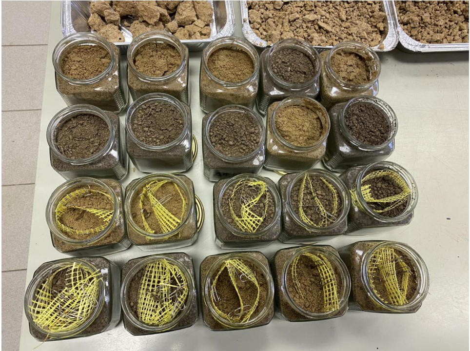
Fig. 5. Soil subsamples in containers and in fruit jars. Upper row, remains of initial soil samples with slightly disturbed (natural) structure. Two rows of jars are for taking aliquots for soil analysis. The two lower rows of jars (with a yellow net) are for putting test objects (linen) to study a cellulolytic activity.
