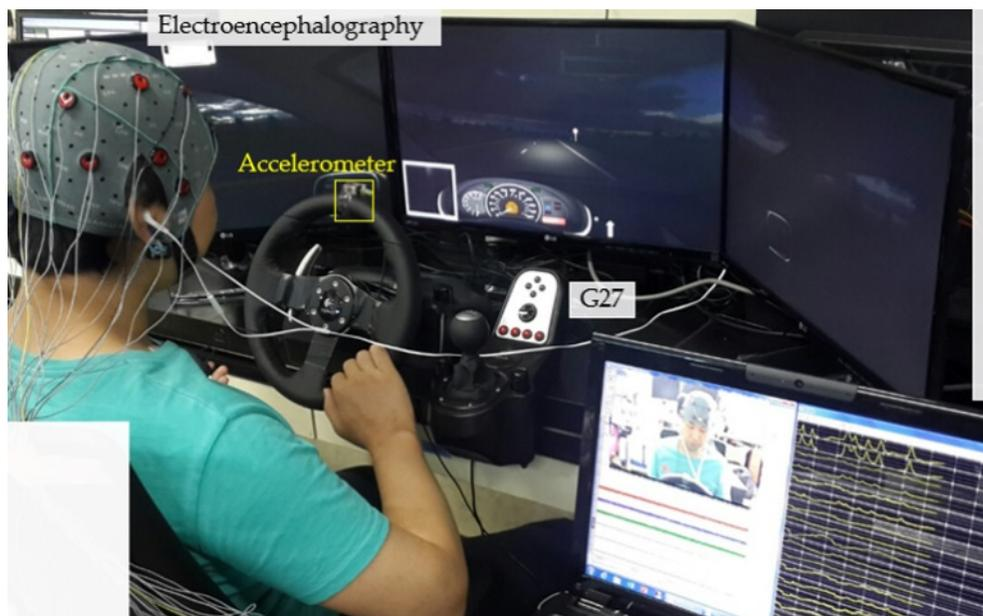
**Figure 1.** Driving simulation with electroencephalogram (EEG) measurements and video recording.
