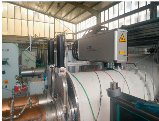
Figure 9. LIBS- system installed at plasma coating device.
