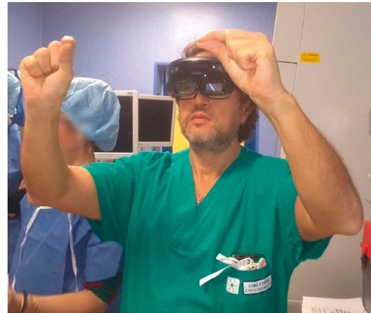
FIGURE 7: Microsoft HoloLens blocks almost 60% of the total light coming from the environment: the wearer's eyes are half-observed by the lenses.
