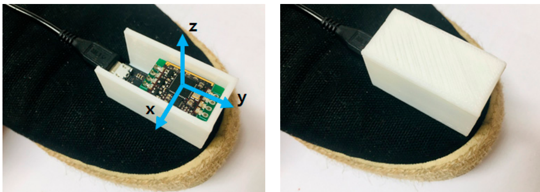
Figure 3. The inertial sensors, in a case made with a 3D printer, are attached to the shoe's tip.
